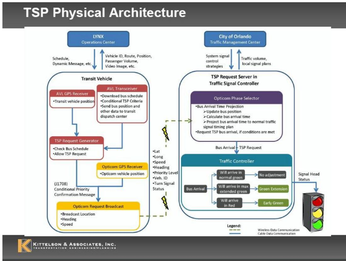
Figure 6: TSP system architecture developed by Kittelson and Associates
