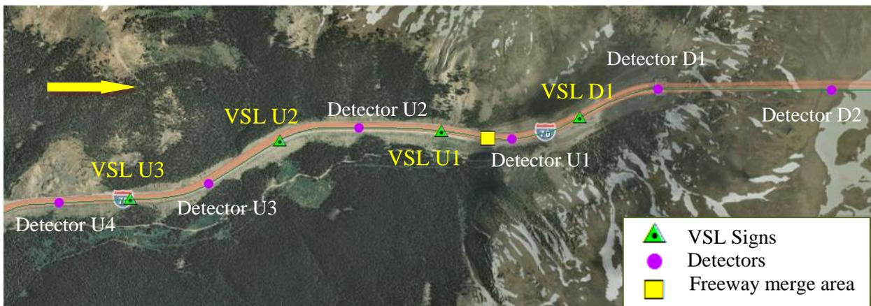
**Figure 6-1: Locations of the VSL signs, detectors and merge point (1:15000)**
