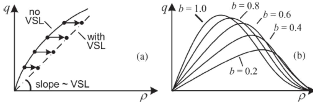
**Figure 3-2(a) Hegyi (2004) model for VSL impact; (b) Cremer (1979) model for VSL impact**
