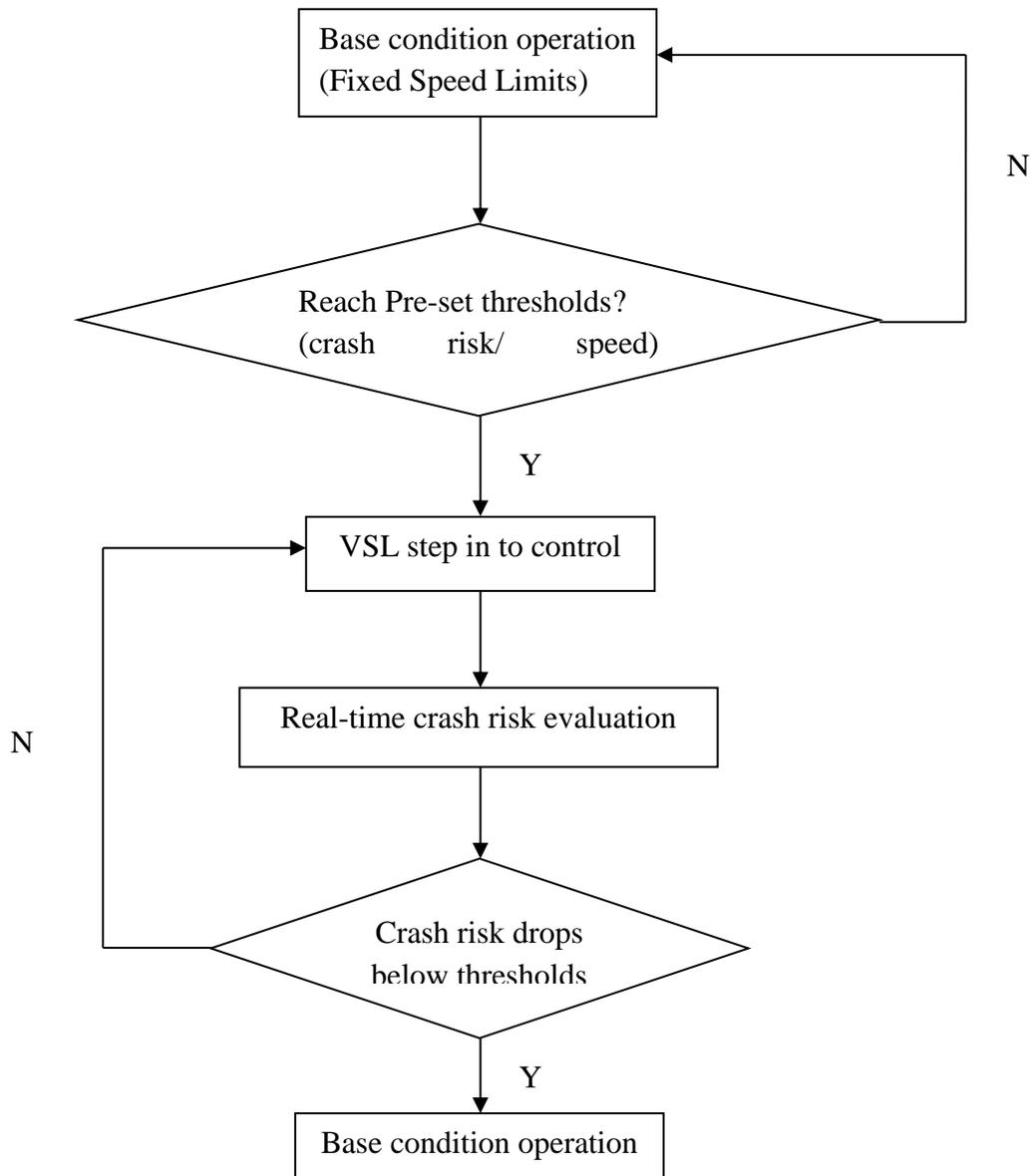
**Figure 3-1 Flow chart of VSL control strategy oriented for traffic safety**
