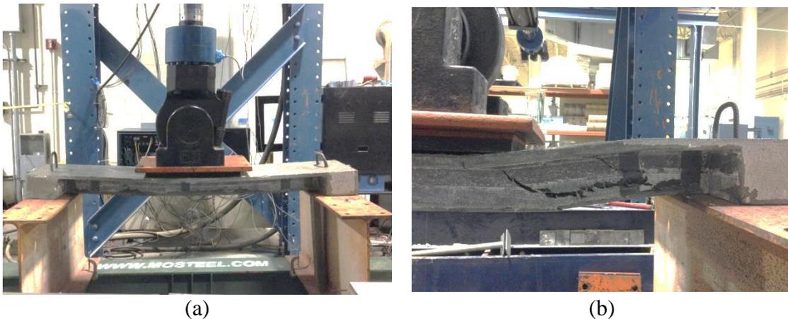
Figure 4.29 Flexure Test and Failure Mode of Specimens 1T1S-HSS, (a) Deflected Shape of Specimen 1T1S, and (b) Beam Shear Crack
