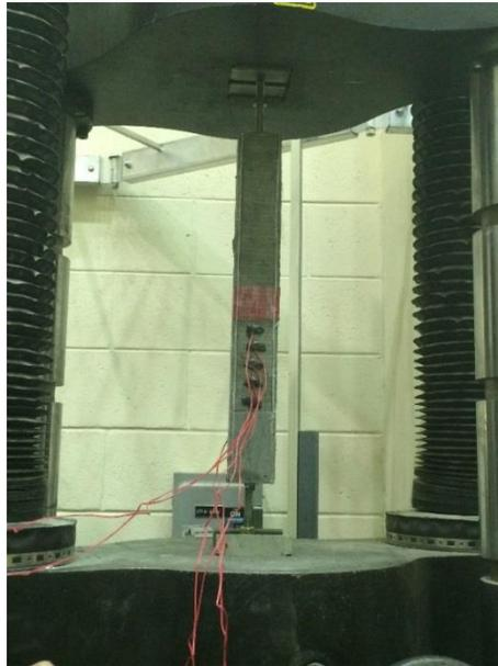
Figure 3.33 Double Lap Specimen Arrangement during the Test
