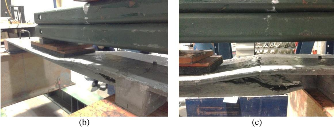
Figure 4.43 Flexure Tests of Specimen 1T2S-HSS: (a) Test Setup, (b) Deflected Shape, and (c) Failure Mode
