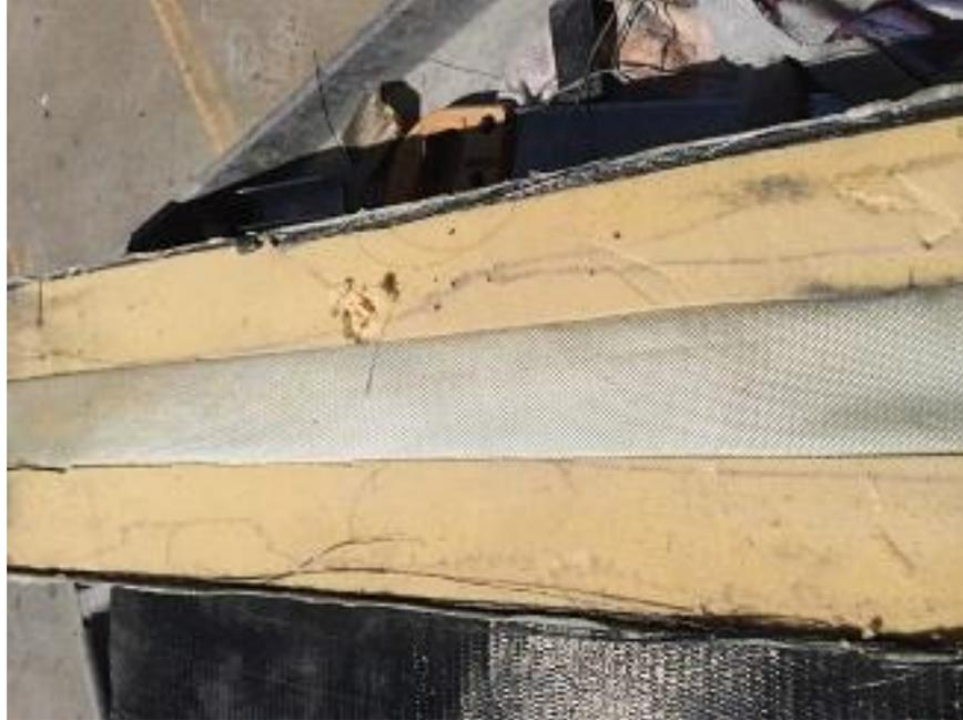
Figure 3.11 The FRP Cloth after Demolding
