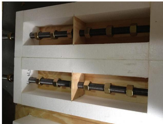
Figure 3.1 Installation and Distribution of High Strength Nuts
