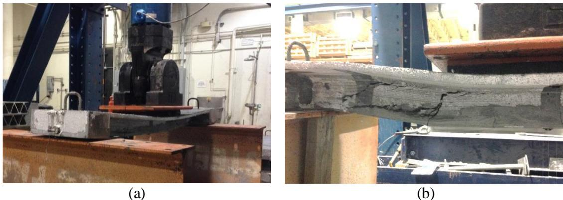
Figure 4.30 Flexure Test and Failure Mode of Specimens 1T1S-CFRP, (a) Deflected Shape of Specimen 1T1S, and (b) Beam Shear Crack
