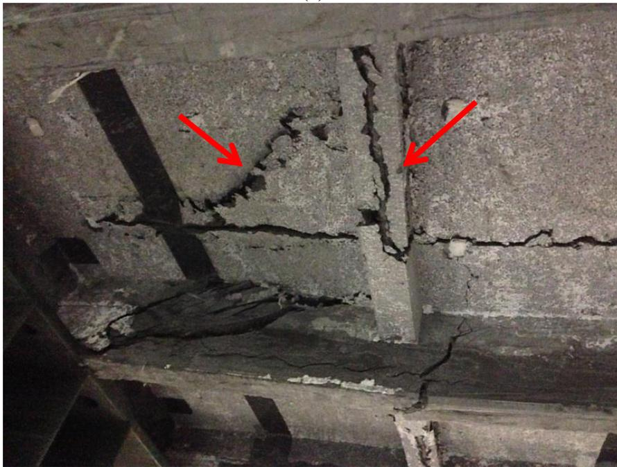
Figure 4.92 Beam Shear Cracks on the Transverse Ribs, (a) FE Modeling, and (b) Experimental Test
