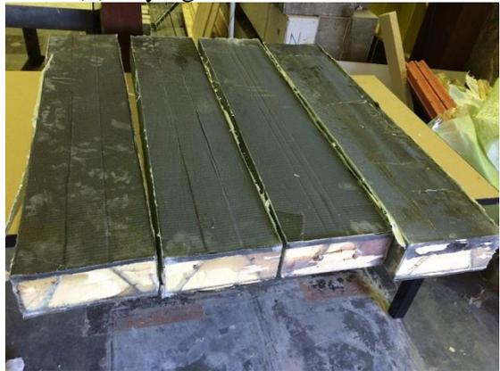
(f) Final Deck after Demolding
