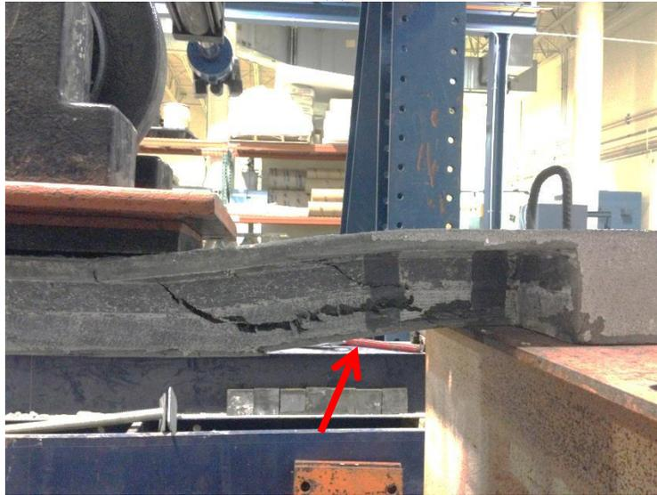
Figure 4.72 Failure Modes and Deflected shape of the Specimen 1T1S-HSS, (a) FE Modeling, and (b) Failure Mode in Experimental Test
