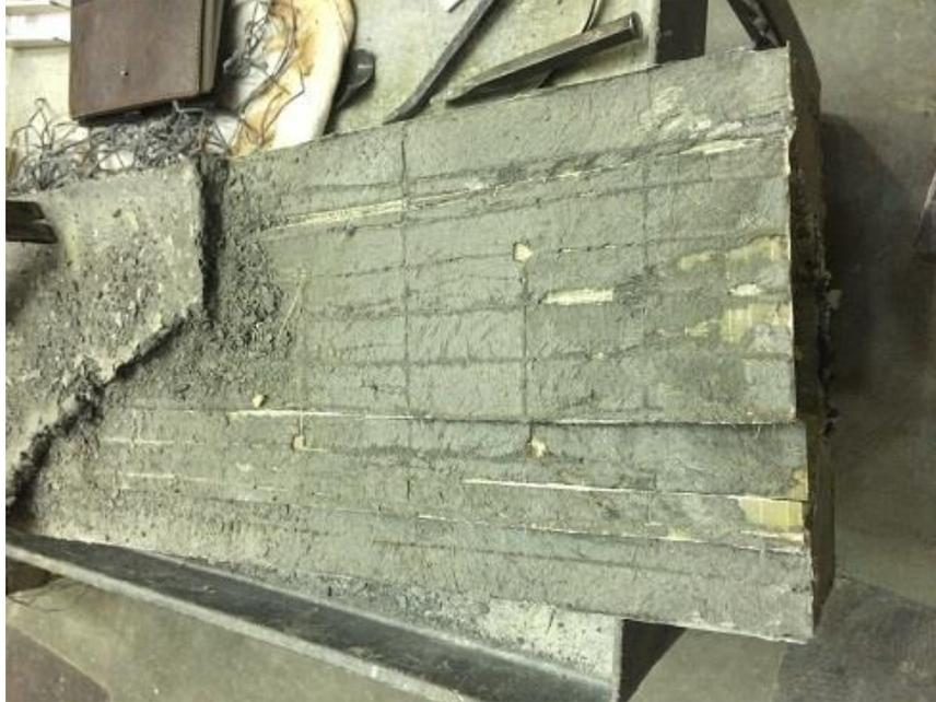
Figure 3.13 The Bond between the UHPC and Top FRP
