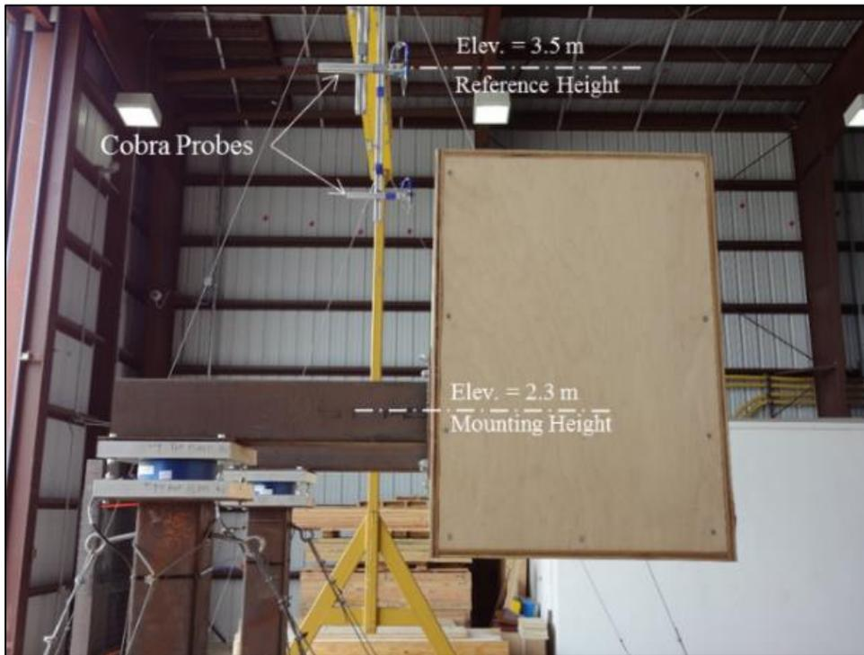
Figure 3.4 Cobra probe configuration (a) looking upstream (b) side elevation
