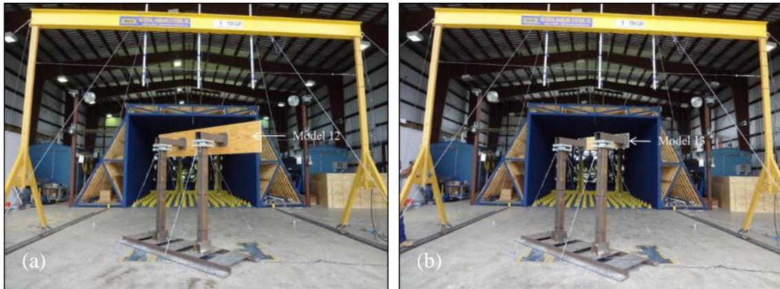
Figure 3.9 Blockage test setup in the WOW (a) 0° configuration (b) 45° configuration
