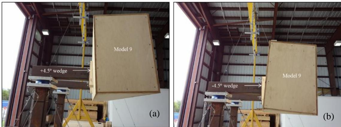
Figure 3.19 Galloping test setup in the WOW (a) Positive  $4.5^\circ$  angle (b) Negative  $4.5^\circ$  angle
