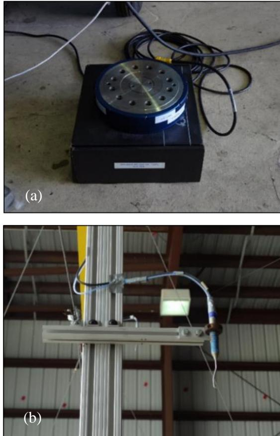
Figure 3.3 Instrumentation (a) JR3 load cell (b) Turbulent Flow Instruments cobra probe
