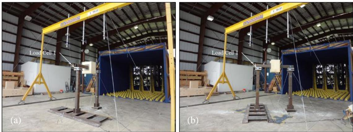
Figure 3.7 Tare test Setup A in the WOW (a) 0° configuration (b) 45° configuration
