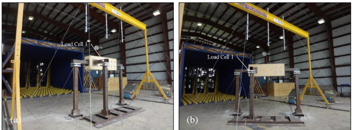
Figure 3.8 Tare test Setup B in the WOW (a) 0° configuration (b) 45° configuration
