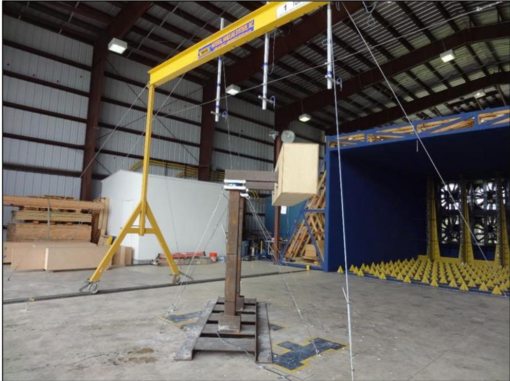
Figure 3.14 Force coefficient test setup in the WOW - 45° wind direction (a) Looking upstream (b) Side view
