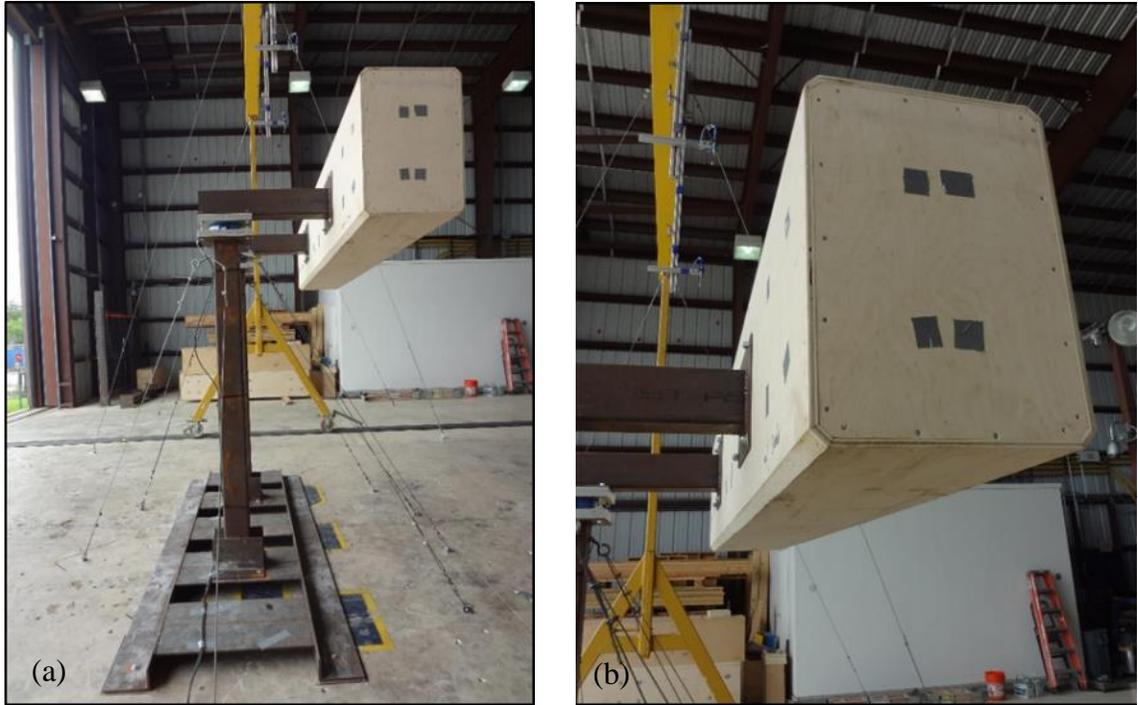
Figure 3.16 Chamfer corner test setup in the WOW (a) Side view (b) Close-up
