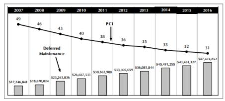
Figure 3: Current Service Level Road Condition and Backlog (1)
