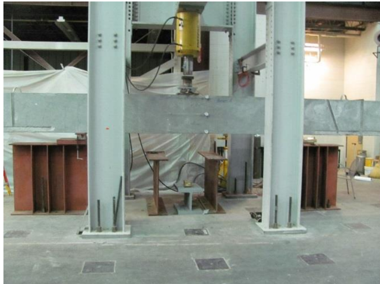
Figure 3.30. Flexural strength test setup.
