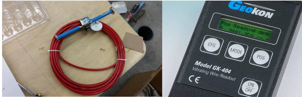
Figure 3.19. Vibrating wire strain gage and readout unit from Geokon
