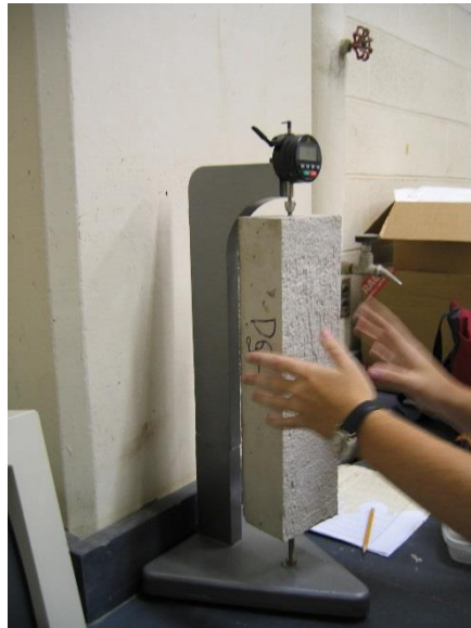
Figure 3.9. Drying shrinkage sample with length comparator
