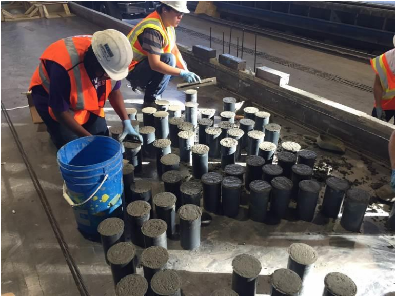
Figure 3.17. Preparation of concrete cylinders for mechanical testing
