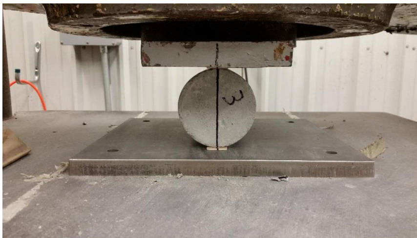
Figure 3.8. Splitting tensile test sample
