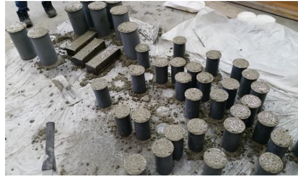
(ii) Concrete filled into molds
