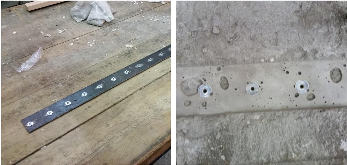
Figure 3.25. Metal nuts for transfer length measurements.
