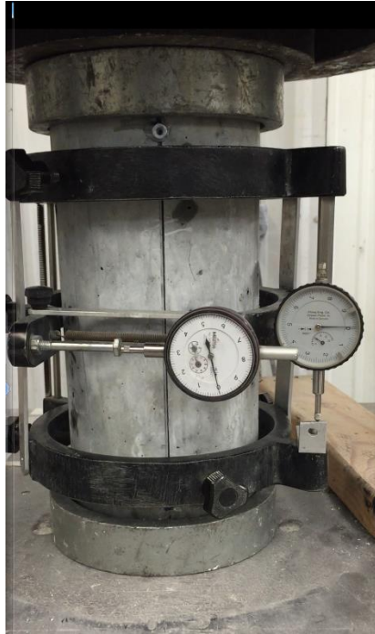
Figure 3.7. Gages for measuring deflections for the Elastic modulus test
