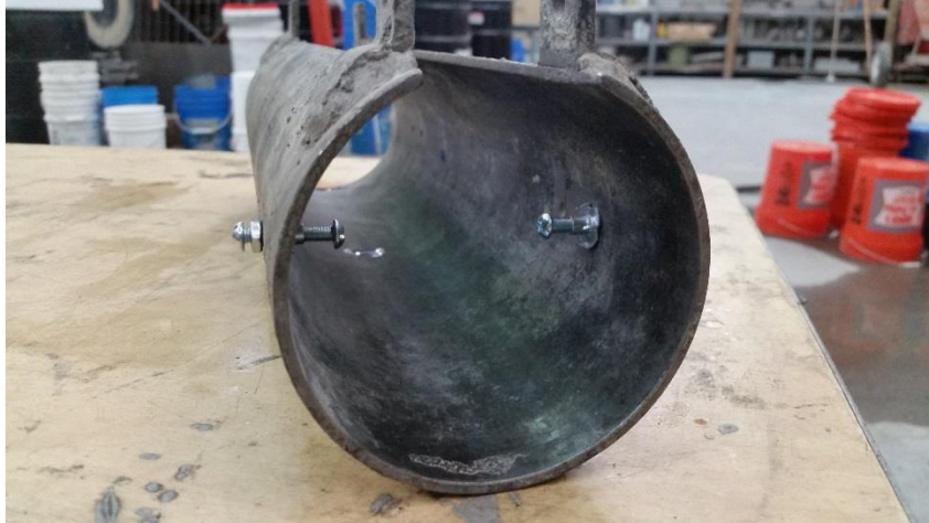
Figure 3.10. Mold used for creep specimens with embedded nuts for DEMEC measurements
