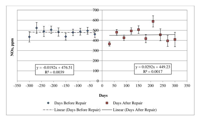
Figure 4-37 NOx measurements 'before' and 'after' repair for vehicles that failed the emission inspection test
