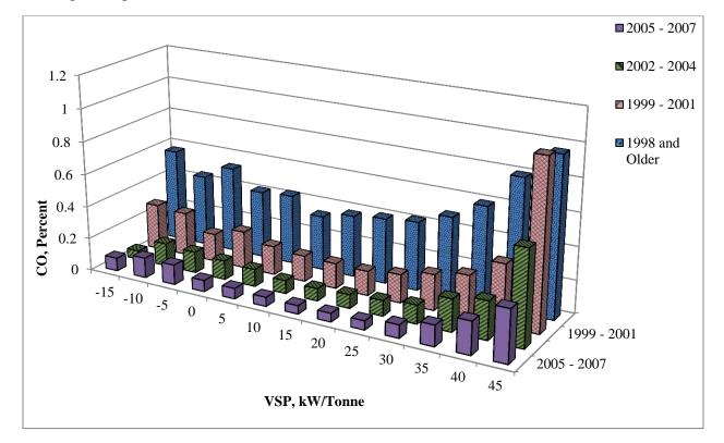
Figure 3-7 Carbon monoxide vs. VSP group by model year
