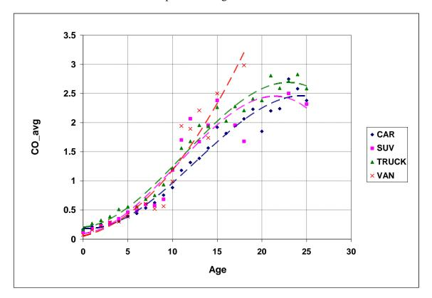
Figure B-5 Age dependence of CO average by model year for various VIN types. Data 1996
