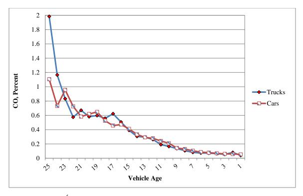
Figure 2-9 CAFÉ 2010 CO emissions vs. vehicle age for car and truck vehicle category
