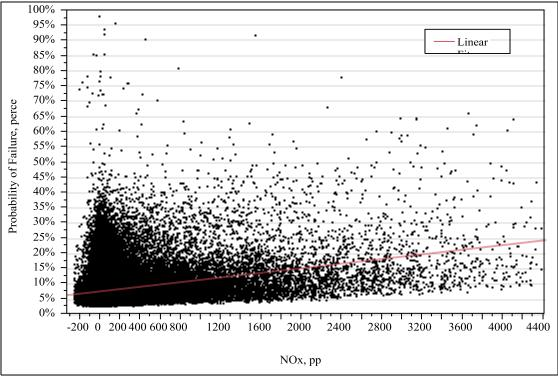
Figure 5-32 Probability of failure vs. nitrogen oxides
