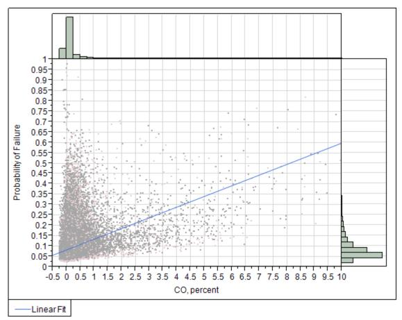
Figure 5-29 Probability of failure vs. carbon monoxide
