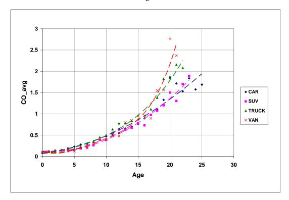
Figure B-6 Age dependence of CO average by model year for various VIN types. Data 2004
