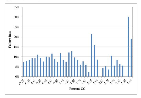
Figure 5-3 Emission test failure rate vs vehicle emission remote sensing carbon monoxide
