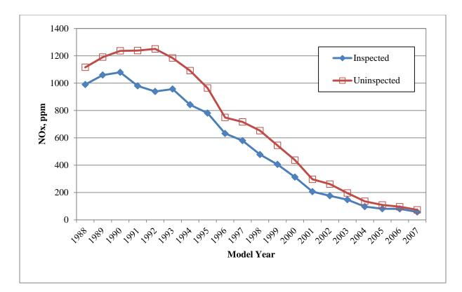
Figure 2-4 Oxides of nitrogen vs. model year for inspected and uninspected fleet
