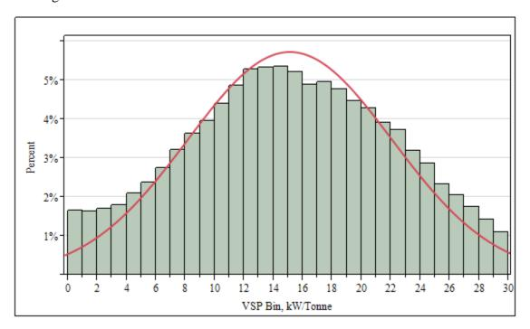
Figure 4-2 Vehicle Specific Power distribution of 'before' emission test sample
