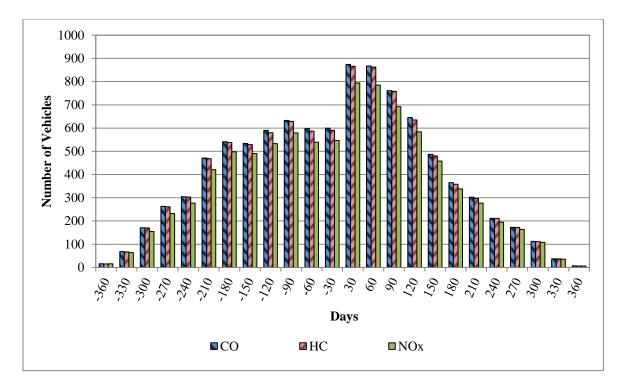
Figure 4-38 Histogram of number of vehicles per bin 'before' and 'after' repair for vehicles that failed the emission inspection test
