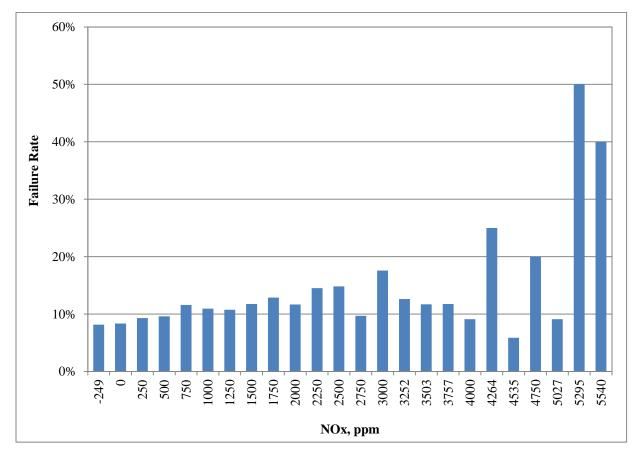
Figure 5-9 Emission test failure rate vs vehicle emission remote sensing nitrogen oxides
