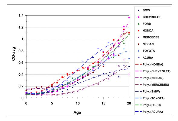
Figure B-2 Dependence of CO average by age for the vehicle makes in the measurement year interval 2005-2008
