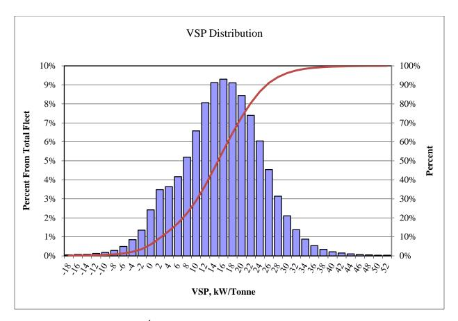
Figure 3-6 CAFÉ 2010 vehicle specific power (kW/Tonne) distribution
