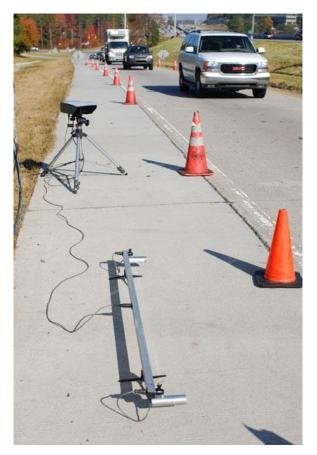
Figure 3-5 Speed Acceleration Bar
