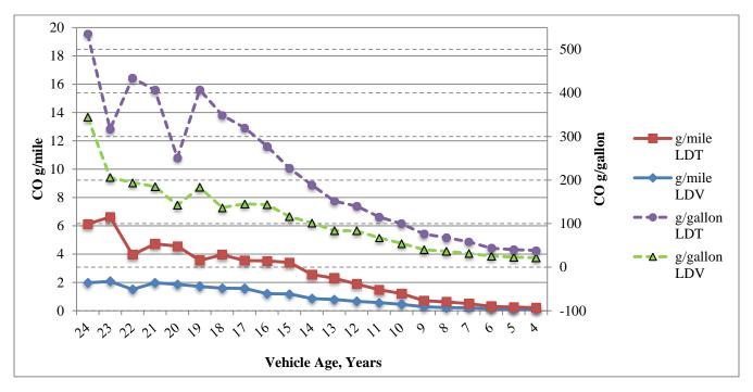
Figure 2-8 Mean CO emissions as a function of vehicle age of RSD CAFÉ 2010 data g/gallon,
