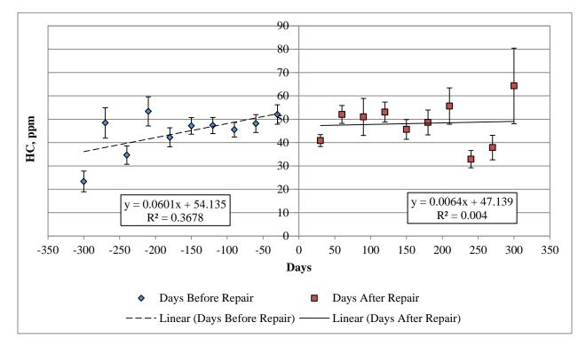
Figure 4-36 HC measurements 'before' and 'after' repair for vehicles that failed the emission inspection test
