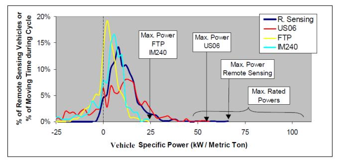
Figure 2-6 Vehicle Specific Power ranges for types of tests
