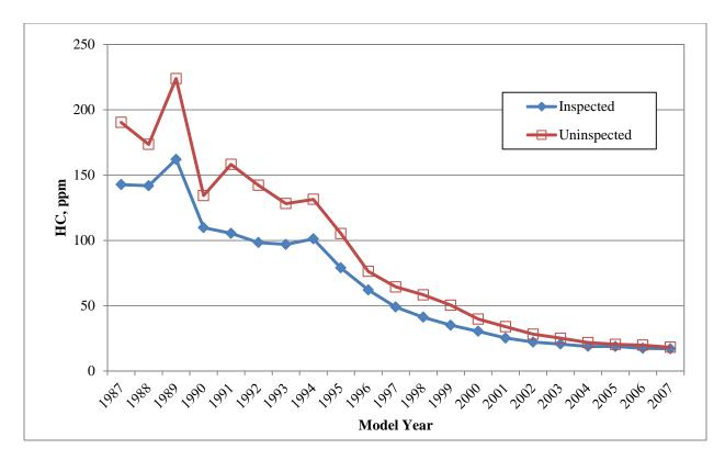
Figure 2-3 Hydrocarbons vs. model year for inspected and uninspected fleet
