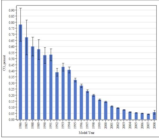
Figure 5-2 Carbon monoxide concentrations vs. model year
