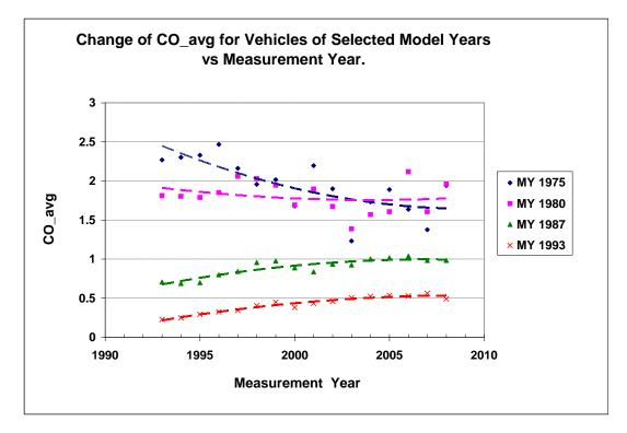
Figure B-11 Change of CO emission from vehicles of various model years by measurement year
