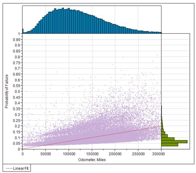
Figure 5-31 Probability of failure vs. odometer readings
