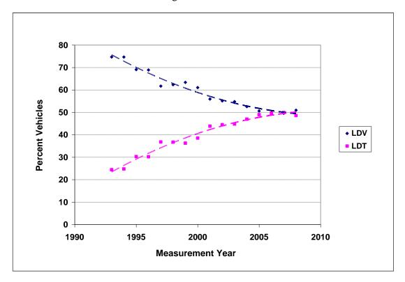
Figure B-4 Percentage of LDV and LDT for various measurement years
