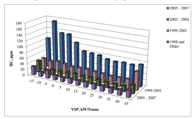
Figure 3-8 Hydrocarbon vs. VSP for model year groups
