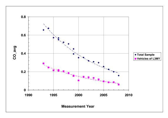
Figure B-8 CO average of total sample and vehicles of latest three model years at various measurement years
