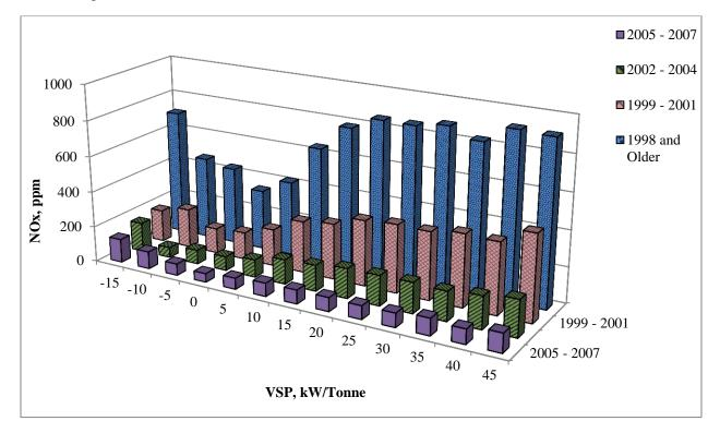
Figure 3-9 Nitrogen oxides vs. VSP for model year groups
