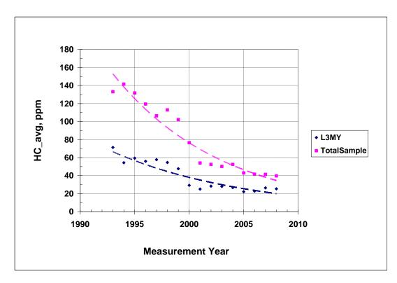
Figure B-9 HC average years sample and vehicles of latest three model years at different
