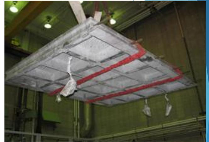
Images taken from full scale laboratory test of UHPC waffle slab bridge deck for Wapello County, Iowa
