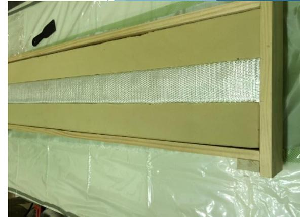
Installing foam and laying shear fiber
