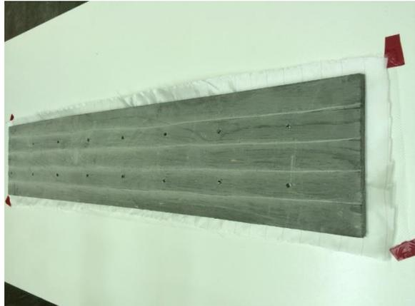
Laying the peel ply, infusion mesh, and UHPC plate
