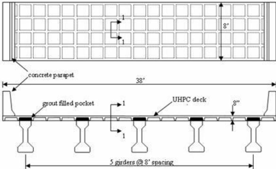
UHPC Two-Way Ribbed Bridge Deck Panel Plan and Cross Section View
