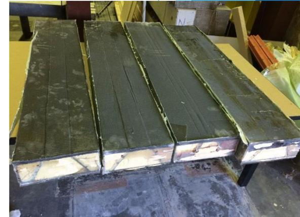
Final deck after demolding
