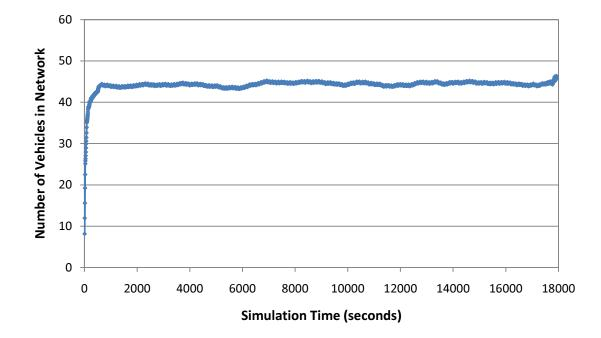
Figure 2. Welch's Method for 5<sup>th</sup> Street Model, window size 100, five hour run
