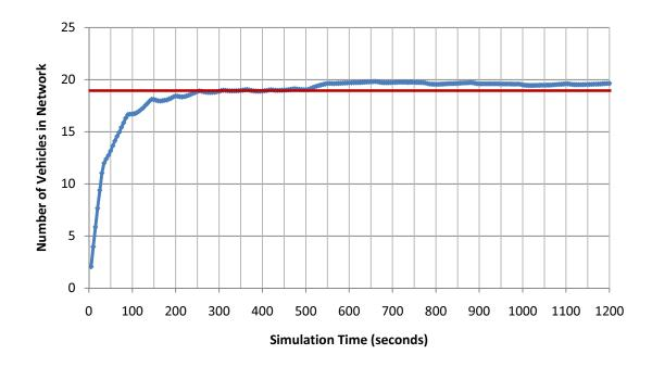
Figure 40. Welch's Method for Identification of warm-up, Small network, 40 replications, w = 100
