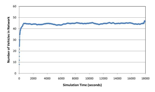
Figure 20. Welch's Method for 20 Replications and window size 100
