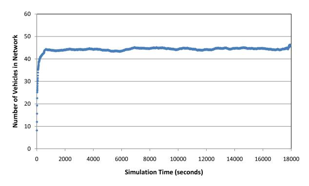
Figure 22. Welch's Method for 40 Replications and window size 100
