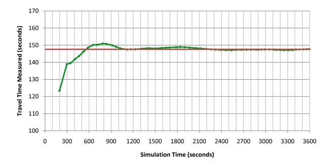
Figure 25. Initial Warm-up of Welch's Method using Travel Time, medium model, 20 replications, w = 50
