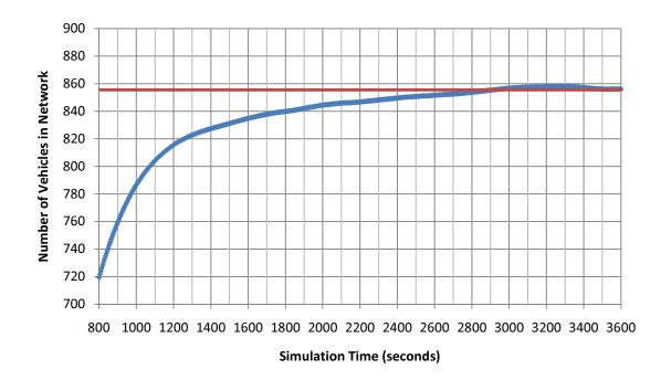
Figure 42. Welch's Method for Identification of warm-up, Large network, 50 replications, w = 150
