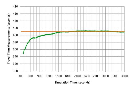
Figure 27. Welch's Method for Travel Times, large model, 40 replications, w = 50
