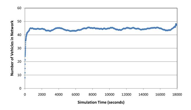
Figure 19. Welch's Method for 10 Replications and window size 100
