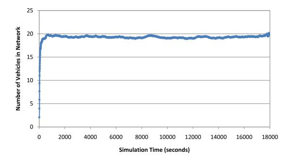
Figure 39. Welch's method for small network, 40 replications, w = 100
