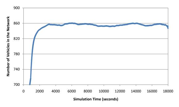
Figure 41. Welch's Method for large network, 50 replications, w = 150
