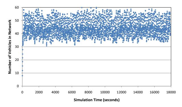
Figure 10. Welch's Method for 10 Replications and a window size 1
