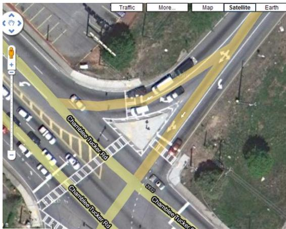
**Figure 46: Ramp Turn Lanes at the Northeast Approach**
