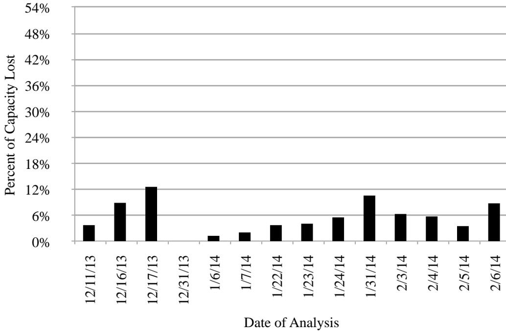
**Figure 68: Percent of capacity lost due to blocking at Peachtree Road & Mathieson Drive.**
