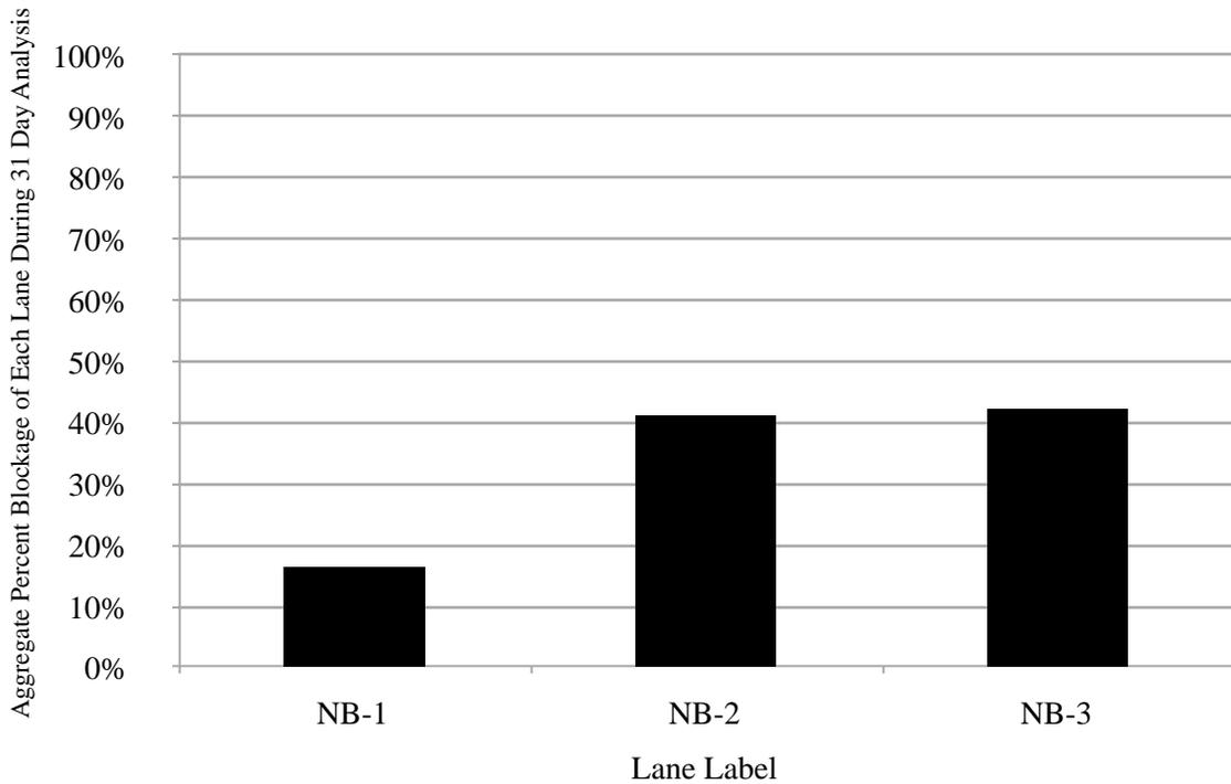
**Figure 78: Aggregate percent of northbound and southbound lanes being blocked at Peachtree Road & Lenox Mall entrance.**
