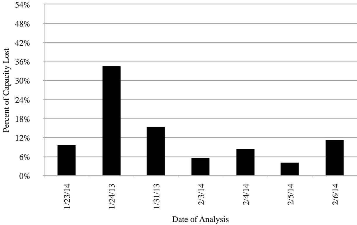
**Figure 70: Percent of capacity lost due to blocking at Peachtree Road & Highland Drive.**
