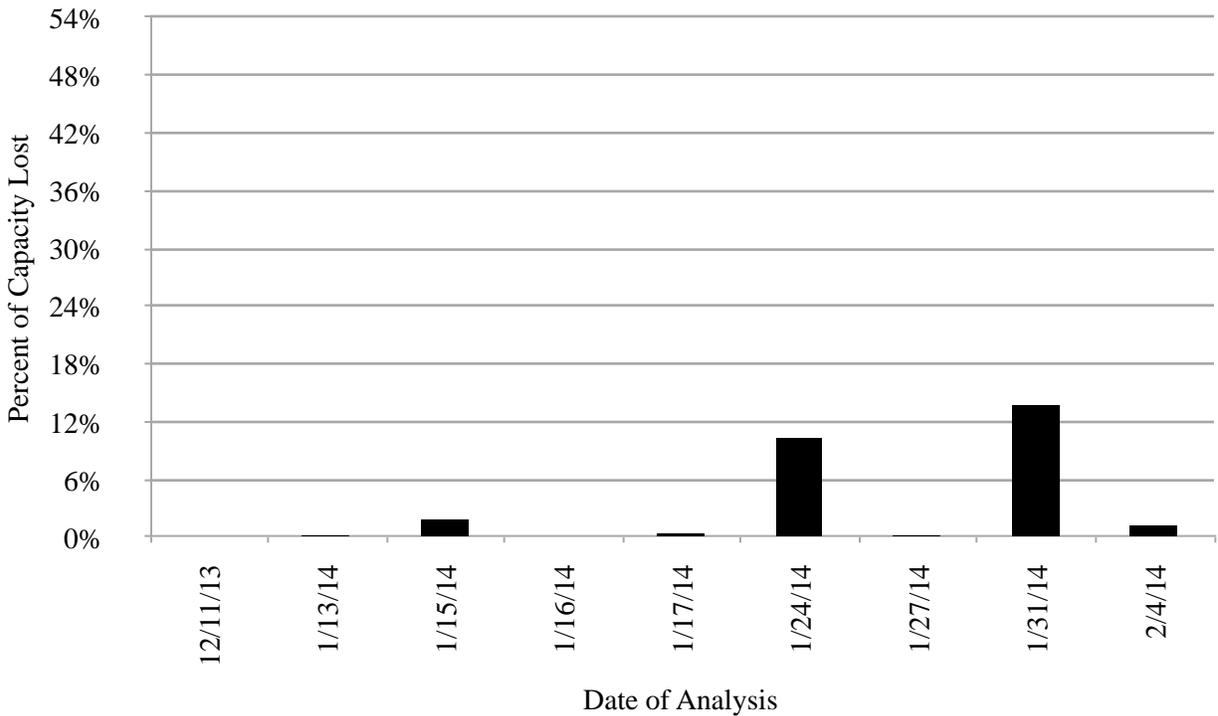
**Figure 69: Percent of capacity lost due to blocking at Peachtree Road & Piedmont Road.**
