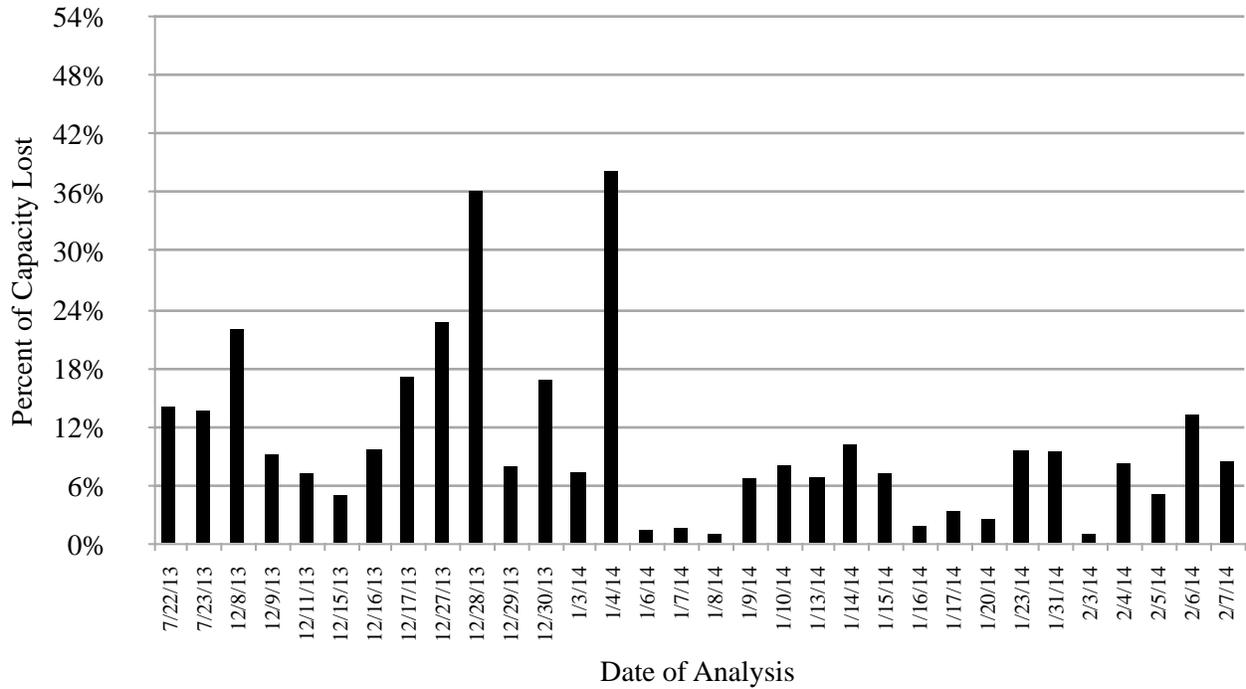
**Figure 72: Percent of capacity lost due to blocking at Peachtree Road & Lenox Road entrance.**
