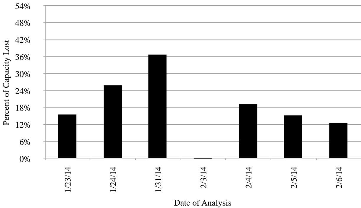
**Figure 71: Percent of capacity lost due to blocking at Peachtree Road & Stratford Road.**
