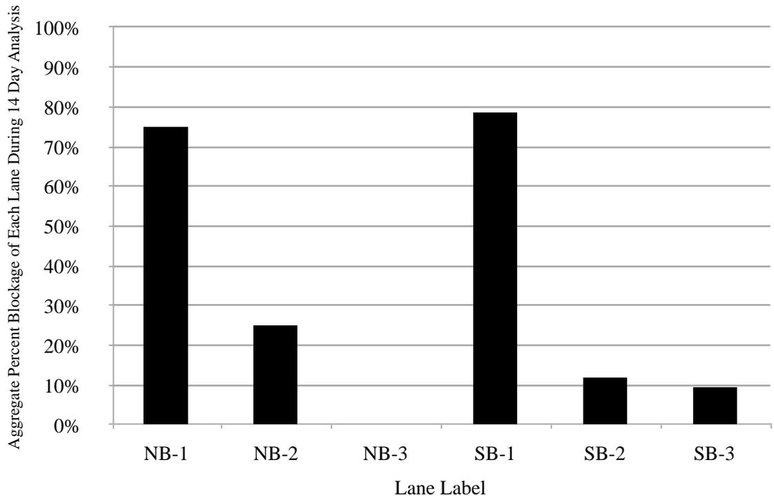
**Figure 74: Aggregate percent of northbound and southbound lanes being blocked at Peachtree Road & Mathieson Drive.**
