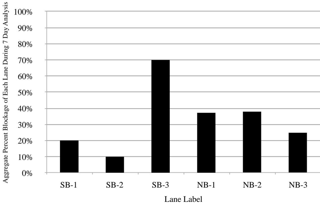
**Figure 77: Aggregate percent of northbound and southbound lanes being blocked at Peachtree Road & Stratford Road.**
